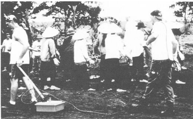
FIG. 1—The radar antenna sled is pulled over the project area that has been stripped of nearly all vegetation. The 500 Megahertz sled (with electronic remote signal) weighs about twelve pounds. It is being used with 60 meters of cable.
